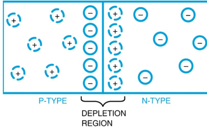
The depletion region is the area near the junction where electrons and holes are depleted; it extends only a short distance on either side of the junction.
